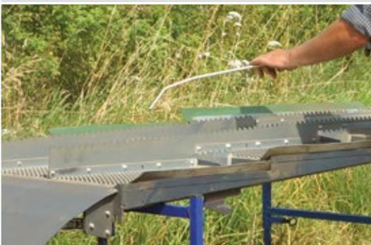
◀ Once removed from the threshing channel, all straw and grain residues can easily and safely be blown away from all components.
