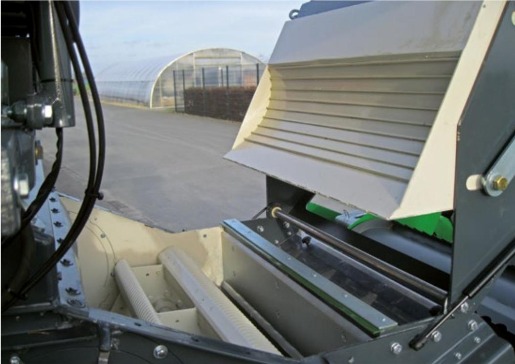
◀ The top-mounted, foldable concave of the ZÜRN 150-EC can be opened in just a few simple steps and offers easy access to the threshing unit within seconds.
