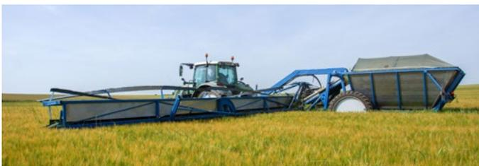
The ZÜRN TOP CUT COLLECT cuts off the top of weed plants and collects the seeds in a bin. This improves field hygiene significantly.
