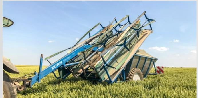
For easy road transport, the booms with up to 18 m working width are folded in hydraulically.
